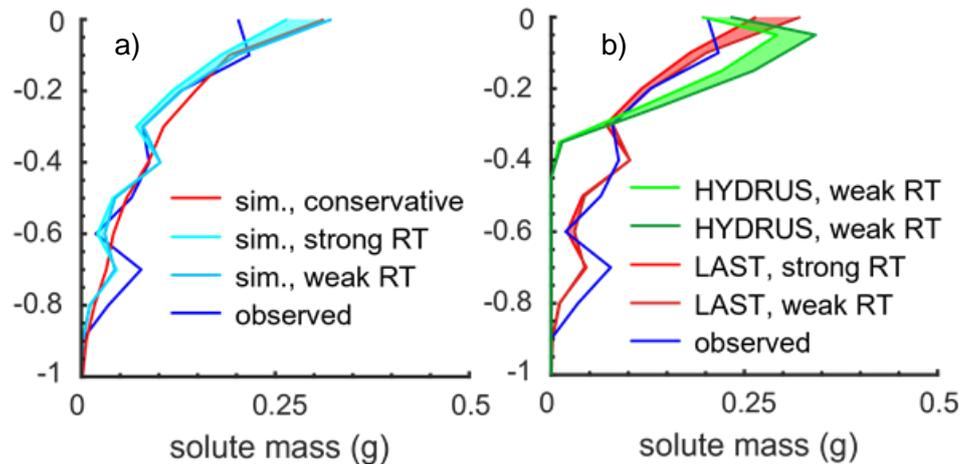
Figure 12: Simulated and observed Isoproturon profiles using LAST at a Weiherbach site dominated by preferential flow (Zehe and Flüßler, 2001) 2 days after application (a), revealing differences in simulated conservative and different reactive transport parametrizations due to the variations of the KF and DT 50 values (RT). Benchmark simulations with Hydrus 1d, shaded areas illustrate the variations of the KF and DT 50 values (b). @ KIT, Sternagel et al. (2021).
