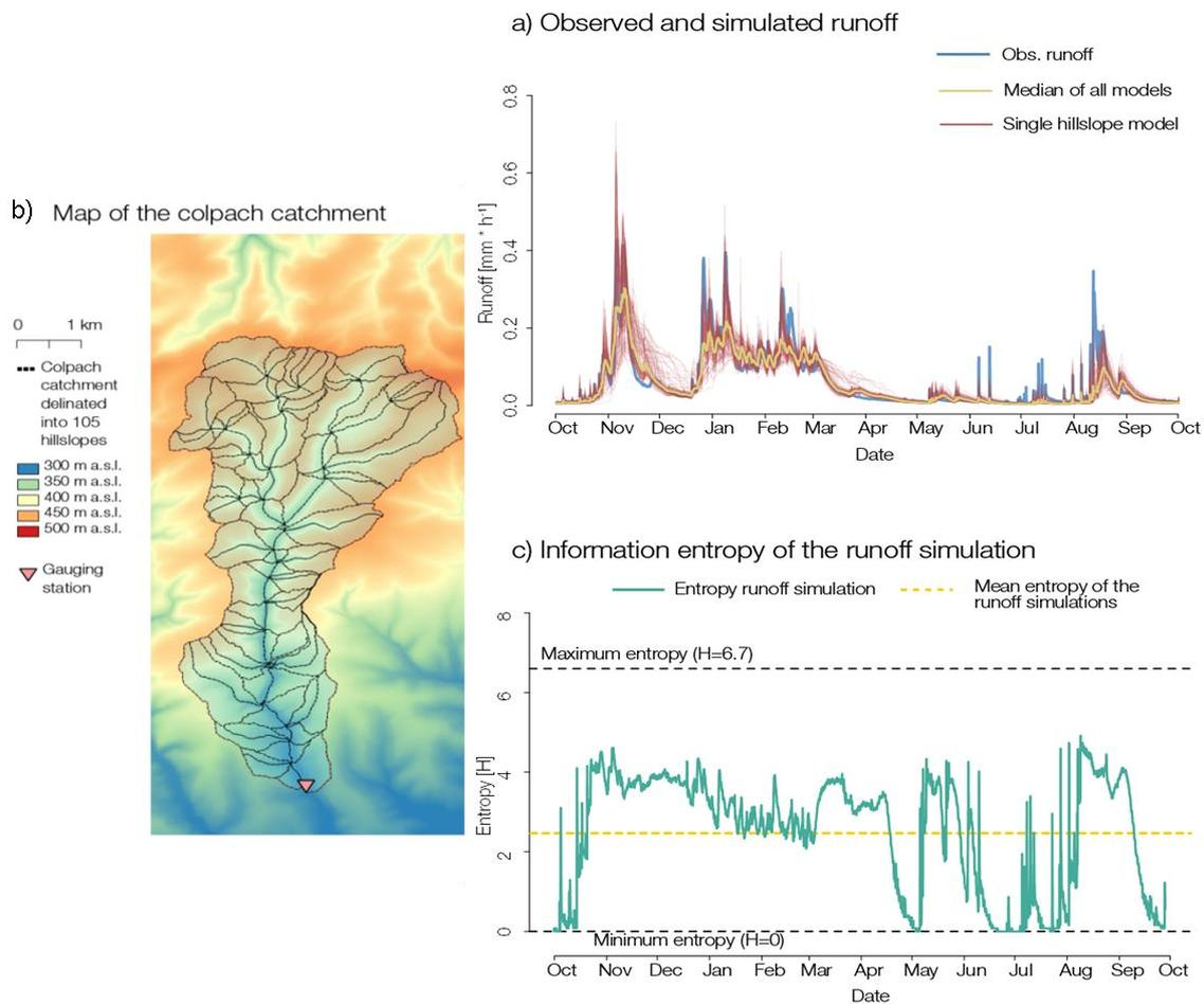
Figure 5: (a) Observed and simulated runoff of the Colpach catchment. The red lines correspond to individual hillslope models and the yellow line to the area-weighted median of all hillslopes. (b) Map of the Colpach catchment and the 105 different hillslopes. (c) Shannon entropy in turquoise for the runoff simulations as well as the corresponding mean. © Ralf Loritz KIT, from Loritz et al. (2018).
