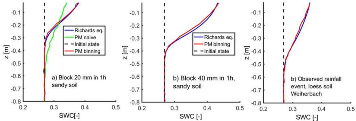
Figure 8: Soil moisture profiles simulated for a) a sandy soil and a block rain of 20 mm with a naive random walk (PM naive) and the Lagrangian particle model with binning (PM) according to Eq. 5 compared to a simulation with a Richards model, b) a sandy soil and a block rain of 40 mm, and c) an observed convective rainfall in the Weiherbach catchment.
