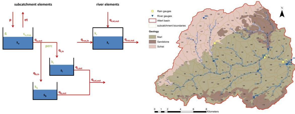
**Figure 5:** Left panel: Structural elements, parameters, state variables and fluxes of the SHM model. Right panel: Attet basin with gauges and SHM sub catchment and river elements.
